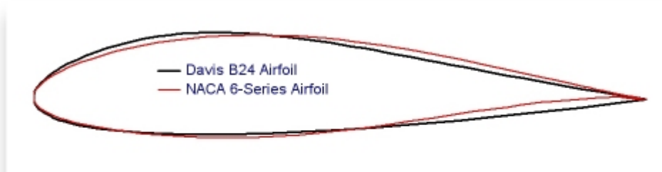
FIGURE 1: An overlay of the Davis airfoil and a similar NACA 6-Series airfoil.
